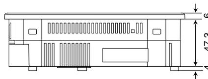
(Note) Since the connection positions of the serial connector CN1 differ when replaced and used from ZM-42 series, it is inconvenient with an attachment space. Be sure to perform a prior check of an attachment position.
