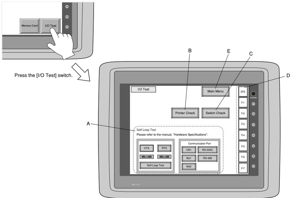
\* In case of ZM-42/43, when the switch "A" on the "Main Menu" is pressed, the following "I/O Test" is displayed.
