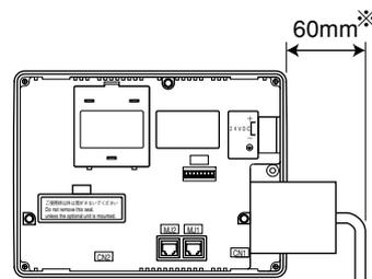
\*60mm is not a size with consideration to the attachment and detachment after attachment. Since it changes in the difference in a wiring system, the electric wire size which wires that check by real wiring
