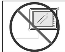
6. Avoid any place in which there is the possibility that water, corrosive gas, flammable gas, solvents or coolants, grinding oil can come in contact with the unit. Never install the unit in a place where dust, salt and metallic particles are present.
