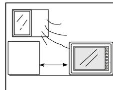
2. Never attach Control Terminal to the top of any apparatus generating high levels of heat (heater, transformer, large-capacity resistor, etc.).
