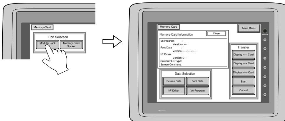
In case of selecting [Memory Card] from [Modular Jack 2] in the [Others] dialog of ZM-71SE, it is possible to select the [Modular Jack 2] switch in the [Port Selection] menu of the [Memory-Card] screen on ZM-\*\*.
