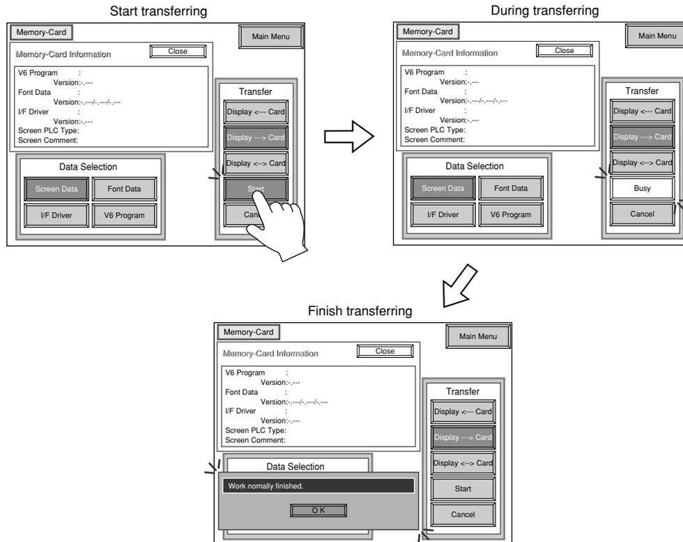
\* When transfer the data from ZM-\*\* to memorycard via the card interface(= [Memory-Card Socket]) of ZM-\*\*, use SRAM type memory card. FROM type memory card is not used.
