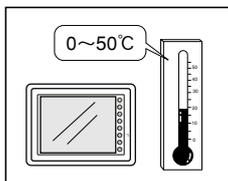
2. Install a forced fan or an air conditioner to maintain the ambient temperature when it is higher than the above mentioned range.
