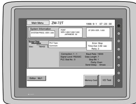
If the screen data has been already transferred to ZM-\*\*, press the [SYSTEM] switch, then press the [F1] switch. The [Main Menu] is displayed.
