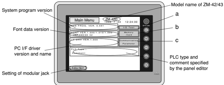
\* In case of ZM-42/43, when the "Communication Parameter" switch on the "Main Menu" is pressed, the following "Comm. Param." is displayed.
